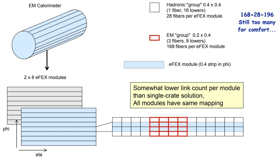
Alternative two crate solution: Cut previous one crate scheme in half at phi=pi with small region needing 1:2 passive optical splitting
