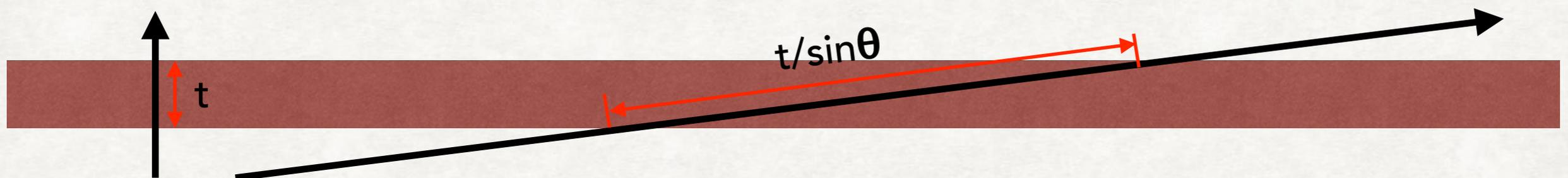
This factor results in choices as to what the optimal way of arranging a detector is. The goal is always to minimise the amount of material i.e. minimise multiple Coulomb scattering that would degrade spatial resolution.
