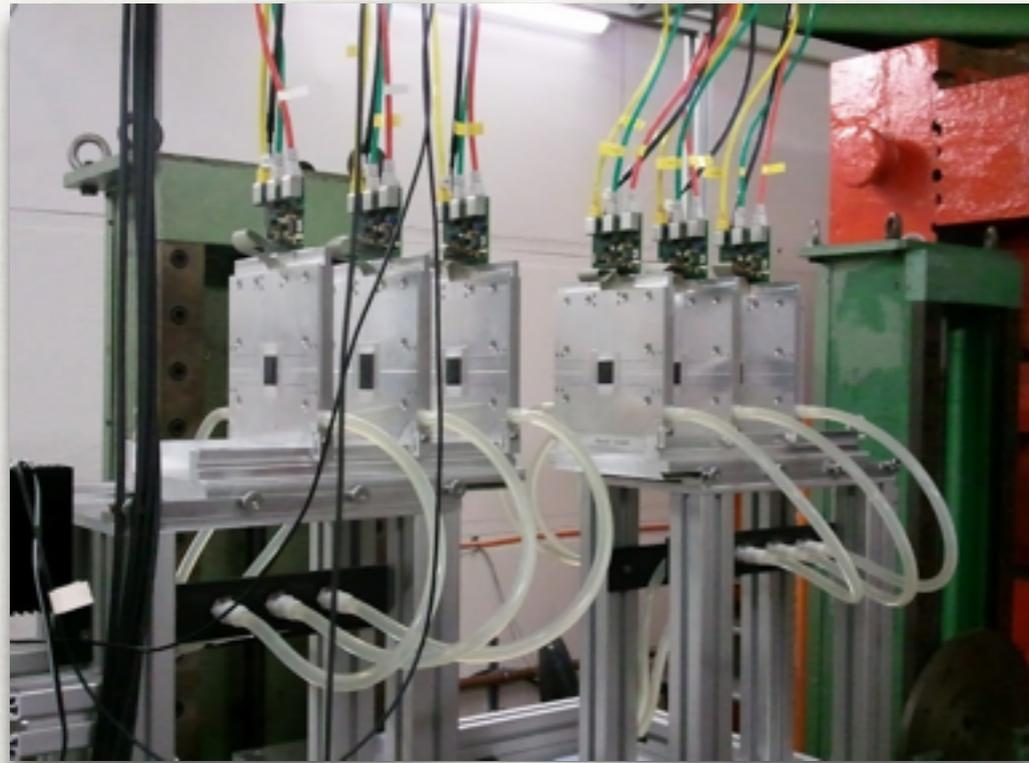
Consists of 6 CMOS sensors from the Mimosa series of chips (developed by the Strasbourg IPHC group).
