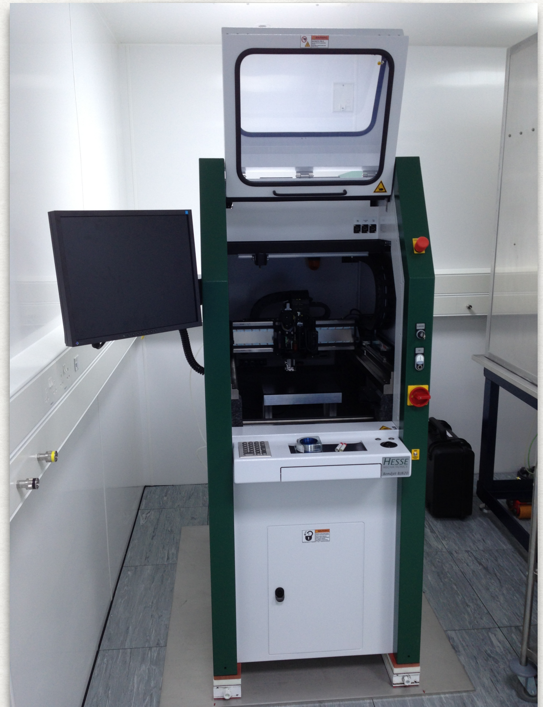
This bonder (Hesse Bondjet BJ820) is used for the ATLAS ITk upgrade at QMUL, and with R&D programmes.
