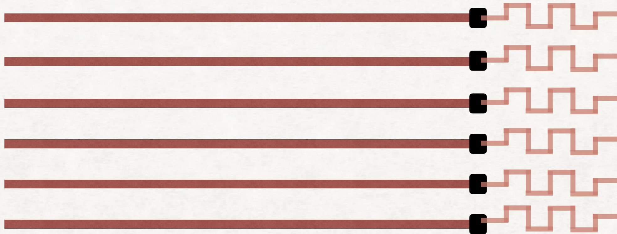
Polysilicon resistor of a few M\Omega to isolate strips from bias
