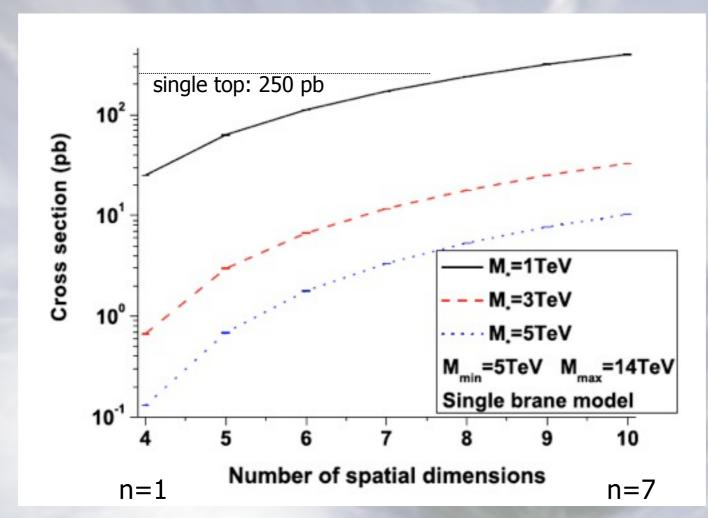
Cross sections vary by  $\sim$  factor 10 for n = 1 $\rightarrow$ 7 Factor  $\sim$ 30 suppression for M<sub>D</sub> = 1  $\rightarrow$  3 TeV
